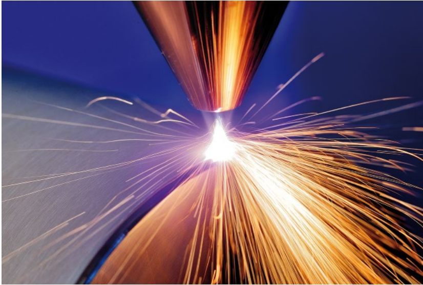
Fig. 7 EHLA: Protection against wear and corrosion, repair and additive manufacturing – all with only one system technology (Source: Fraunhofer ILT)
