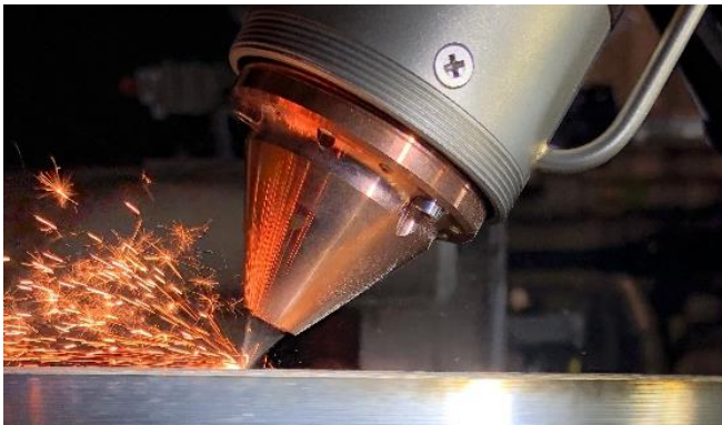
Figure 1: Extreme High-speed Laser Material Deposition (EHLA) with a HighNo powder nozzle in 30° © HD Special Optics for Laser Technology and Fraunhofer ILT
